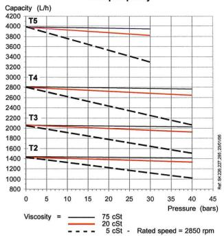
Data shown are for new pumps, with no allowance for wear.
