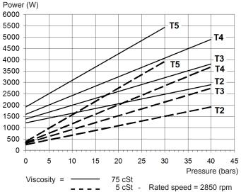
Data shown are for new pumps, with no allowance for wear.
