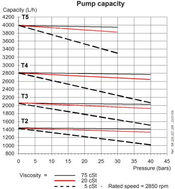
Data shown are for new pumps, with no allowance for wear.
