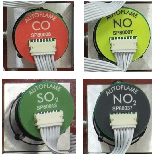
Figure 3.8.2.i CO, NO, SO 2 and NO 2 Cells
